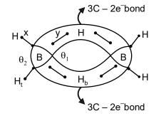
$B_2H_6$  have 4 2c-2e bonds and 2 3c-2e bonds. Bridging bonds have larger bond length than terminal bonds. Angle between terminal bonds in more than angle between bridging bonds if all 4 terminal bonds are in one plane then bridging bonds are in perpendicular plane.
